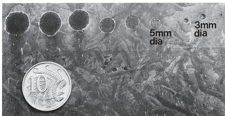
The galvanized steel test piece has had circular areas of the coating removed before exposure in a severe industrial environment. Sacrificial protection is provided by the surrounding galvanized coating and has prevented corrosion of the exposed circles up to 3mm diameter and minimised corrosion of the 5mm circle. Larger circles also exhibit corrosion-free annular areas adjacent to the surrounding coating.
